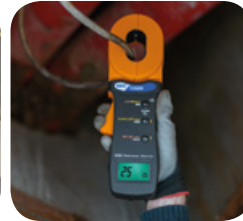
Earth resistance measurement with clamp T2100.
