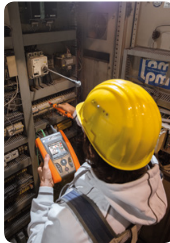
Start/stop measuring with remote lead PR400.
