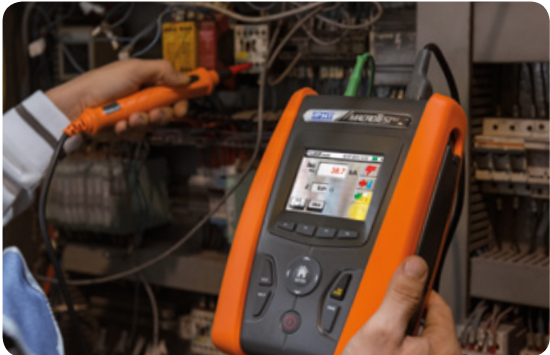
Start/stop measuring with remote lead PR400.
