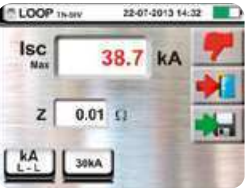
Negative result of breaking capacity test.
