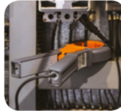
Measurement of leakage current with optional clamp HT96U.
