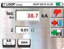
Advanced Loop: negative result of breaking capacity test.
