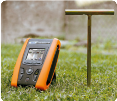
Measurement of earth impedance by voltammetric method.
