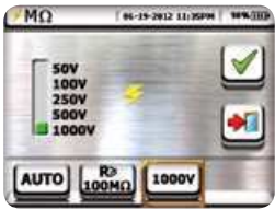
Selection of test voltage and minimum limit value on MΩ measurement.
