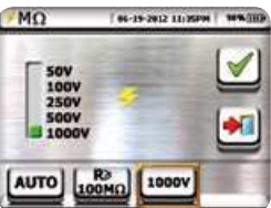
Selection of test voltage and minimum limit value on measurement.
