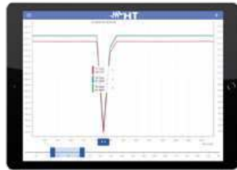
Example of display Recording made (evident voltage interruptions)
