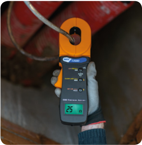
Measurement of earth resistance with Clamp T2100.
