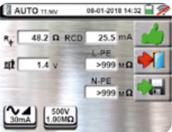
Autosequence: automatic sequence of measurements of Overall earth resistance, RCD test and Insulation L-PE, N-PE.
