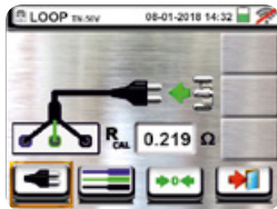
Zero-loop: compensation of the resistance of the test cables used for Loop impedance measurement.
